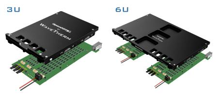
Note: 6U Assembly has two separate PCBs that should be wired independently.
