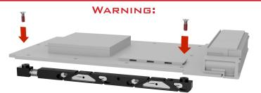
SOLIDWEDGEs are not intended to be mounted directly to PCBs. The opposing force of the mounting blocks may result in board damage.
