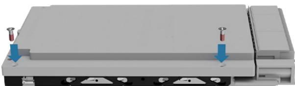
Install screws and torque to 2 in-lbs. Ensure mounting screw doesn't hit drive screw.
