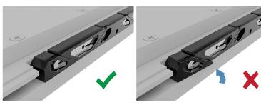
Check alignment on both mounting blocks after torquing and press to straighten if necessary.
