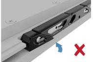
Check alignment on both mounting blocks after torquing and press to straighten if necessary.
