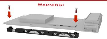
SOLIDWEDGEs are not intended to be mounted directly to PCBs. The opposing force of the mounting blocks may result in board damage.
