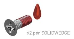
Apply Loctite 2760 to #2-56-100° flat head mounting screws (not included)
