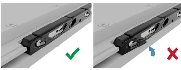
Check alignment on both mounting blocks after torquing and press to straighten if necessary.
