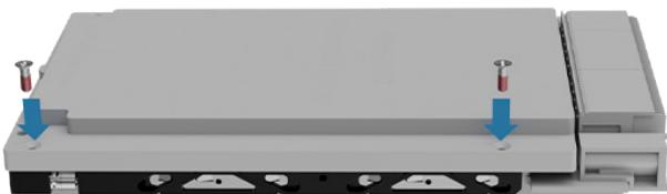
Install screws and torque to 2 in-lbs. Ensure mounting screw doesn't hit drive screw.
